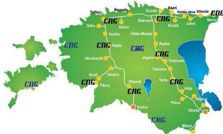
Optimal location of CNG filling stations (black – close to natural gas grid, blue – off the natural gas grid, either biomethane or natural gas from LNG terminal will be used).
