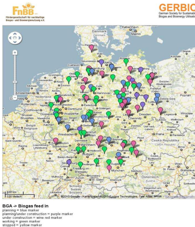
Biogas plants with upgrading and feed-in to the natural gas grid (GERBIO)
