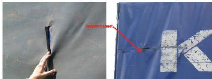
B: Sheet ripped during journey, with minor damage. Dependent on the commodity being transported, this trailer COULD be allowed to complete the current journey - but should NOT be able to carry out further international transport without being repaired.
