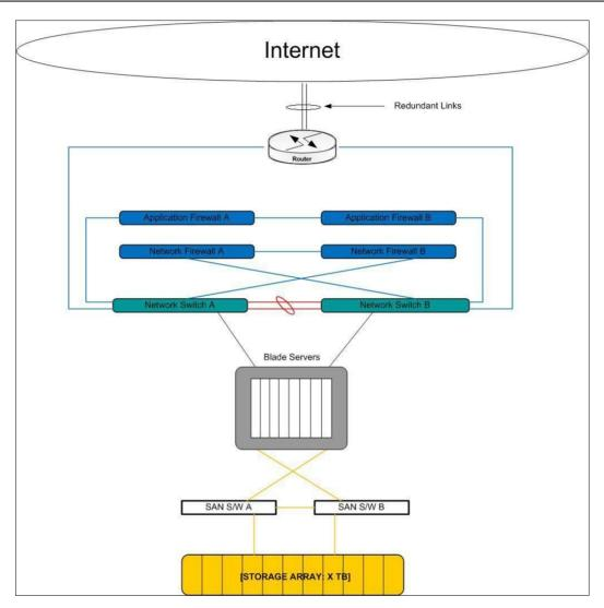
Figure 2-4: The Blade Center Configuration
