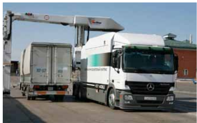
A Russian mobile cargo inspection unit at work.
