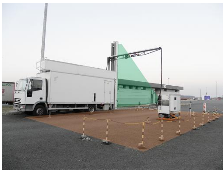
Picture 3 – Silhouette scanner type – 300 keV transmission x-ray unit, continuous exposure. Exclusion zone around the full operational unit is shown.
