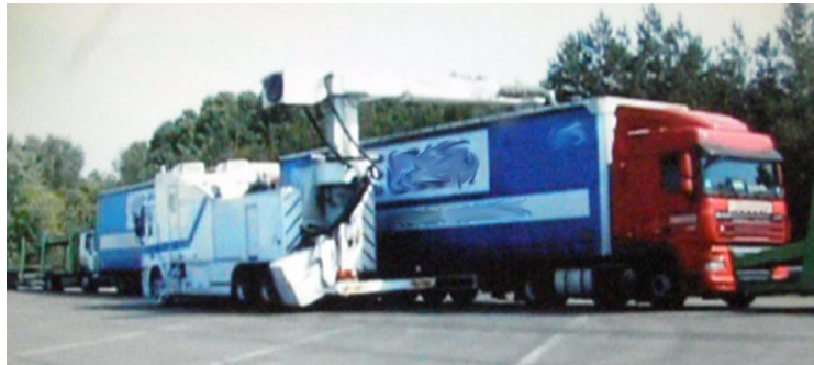
Picture 5 – LINAC, high-energy x-ray scanning unit (type – 4.5 MeV pulsed exposure) scans the properly lined queue of vehicles.
