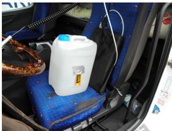
Picture 1 – Water phantom, representing the driver and dosimeter on the driver seat in the scanned truck cabin.
