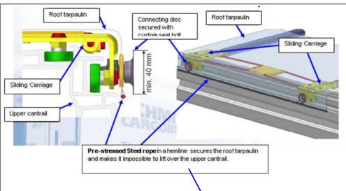
With additional connecting discs (200mm) it is not possible to open the roof to a maximum.
