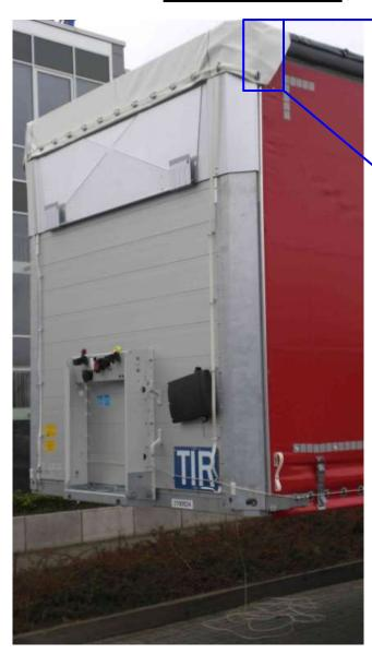
The fixing point of the fastening steel rope is completely covered and secured by the roof curtain.
