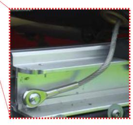
Detail photo from the fixing point of the fastening steel rope at the front.
