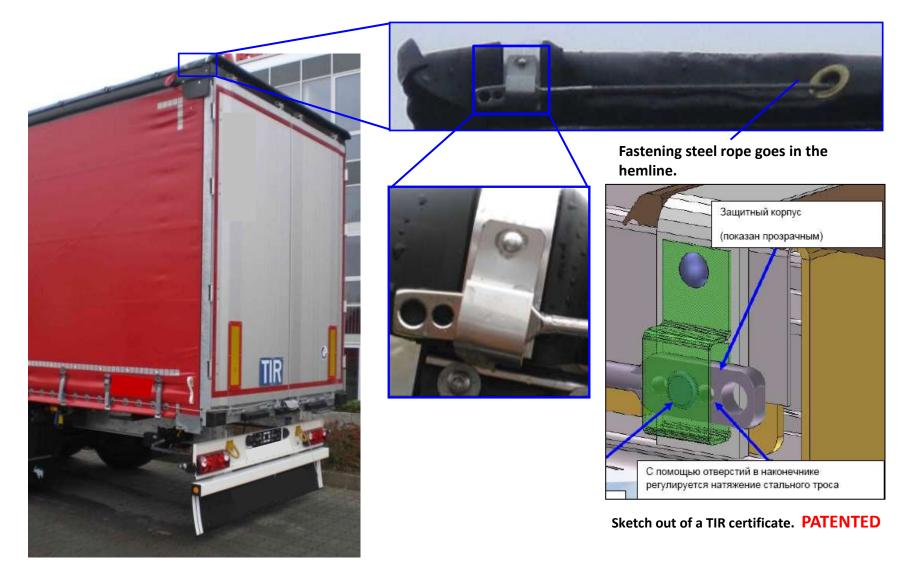
Due to the fact that there are certainly other solutions to secure the fastening steel rope and that this system is patented from a manufacturer, this system should not be described in the TIR Handbook. If the WP30 do though, then only as example and with the remark PATENTED.
