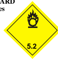
(No 5.2) Symbol (flame over circle): black; Background: yellow; Figures '5.2' in bottom corner
