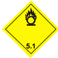
(No 5.1) Symbol (flame over circle): black; Background: yellow; Figures '5.1' in bottom corner
