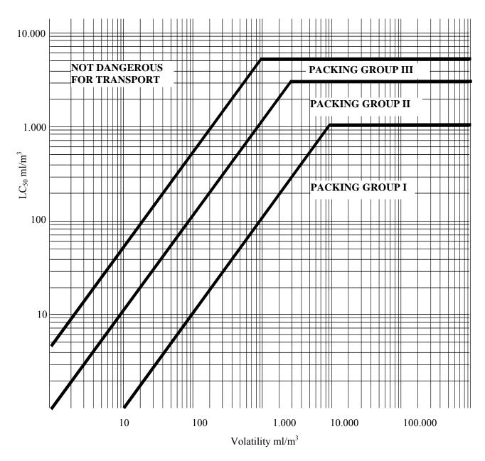
In this figure, the criteria are expressed in graphical form, as an aid to easy classification. However, due to approximations inherent in the use of graphs, substances falling on or near group borderlines shall be checked using numerical criteria.
