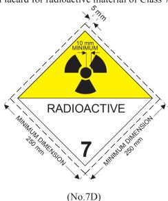
Symbol (trefoil): black; Background: upper half yellow with white border, lower half white; The lower half shall show the word "RADIOACTIVE" or alternatively the appropriate UN Number and the figure "7" in the bottom corner.
