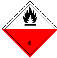
(No.4.2) Division 4.2 Substances liable to spontaneous combustion Symbol (flame): black; Background: upper half white, lower half red; Figure '4' in bottom corner
