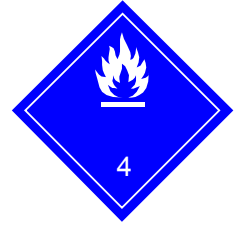
(No.4.3) Division 4.3 Substances which in contact with water emit flammable gases Symbol (flame): black or white; Background: blue; Figure '4' in bottom corner
