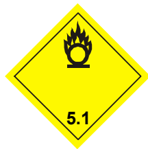
(No. 5.1) Division 5.1 Oxidizing substances Symbol (flame over circle): black; Background: yellow; Figures '5.1' in bottom corner
