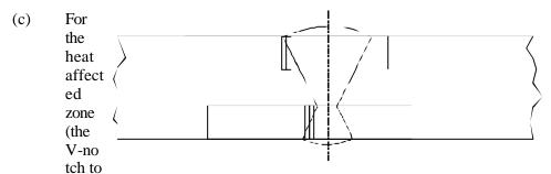
cross the fusion boundary at the centre of the specimen) the value obtained from not more than one of the three test-pieces may be below the minimum value of 34 J/cm<sup>2</sup>, though not below 24 J/cm<sup>2</sup>.
