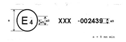
The above approval mark affixed to a vehicle shows that the vehicle type concerned has, with regard to its heating system(s), been approved in the Netherlands (E 4) for Class III, pursuant to Regulation No. XXX. The number 00 indicates that the approval was granted according to the requirements of Regulation No. XXX in its original form.
