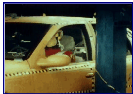
Figure 6 -- Side impact pole test
