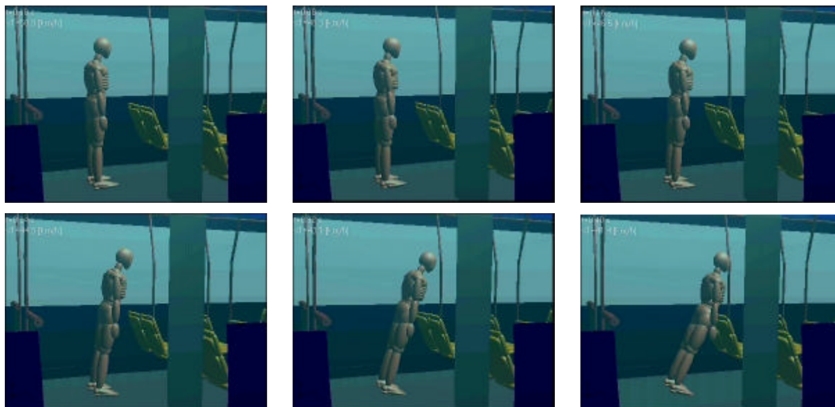
Figure 77 - 50 th percentile H III dummy standing in front of a vertical grab rail at 80ms intervals
