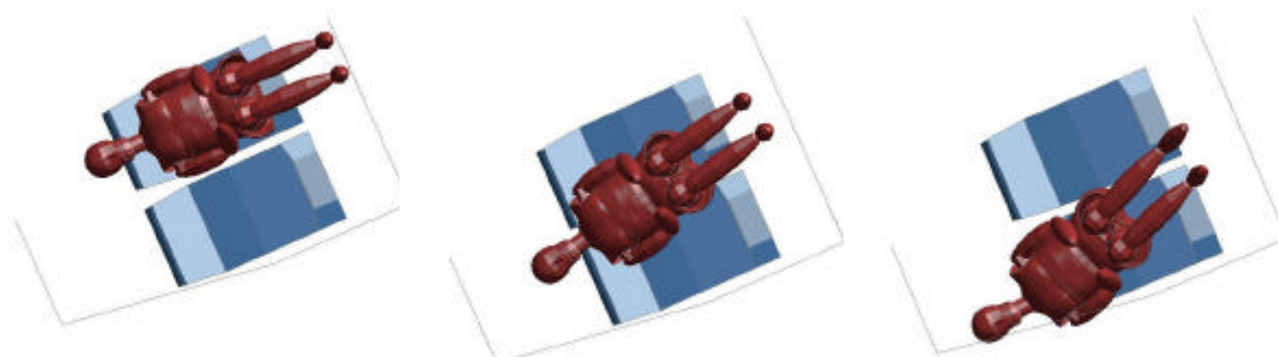
Figure 42 - Kinematics of unbelted M2 rollover occupant model seated away from sidewall (t = 0, 100 and 200ms).
