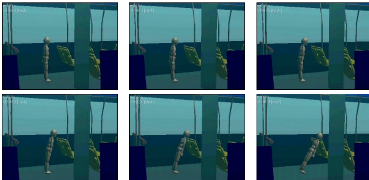
Figure 80 - 6 year child dummy standing in front of a vertical grab rail 80ms intervals
