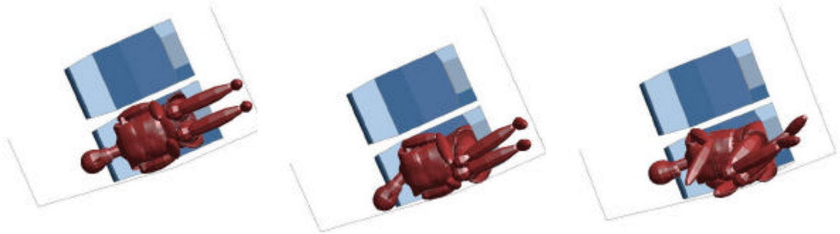
Figure 41 - Kinematics of M2 rollover occupant model seated next to sidewall with increased stiffness properties (t = 0, 100 and 200ms).
