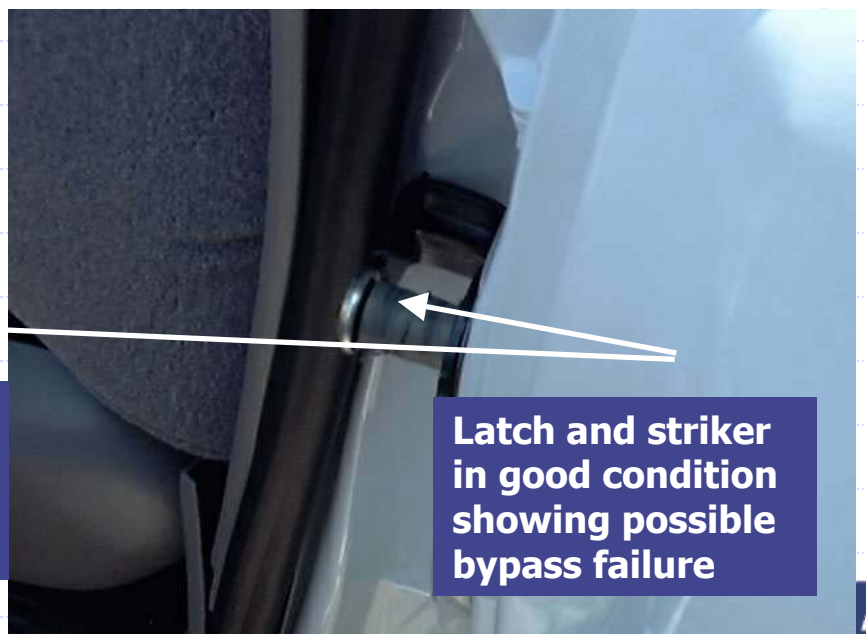
Separation between the door and pillar shows rearward displacement of the door
