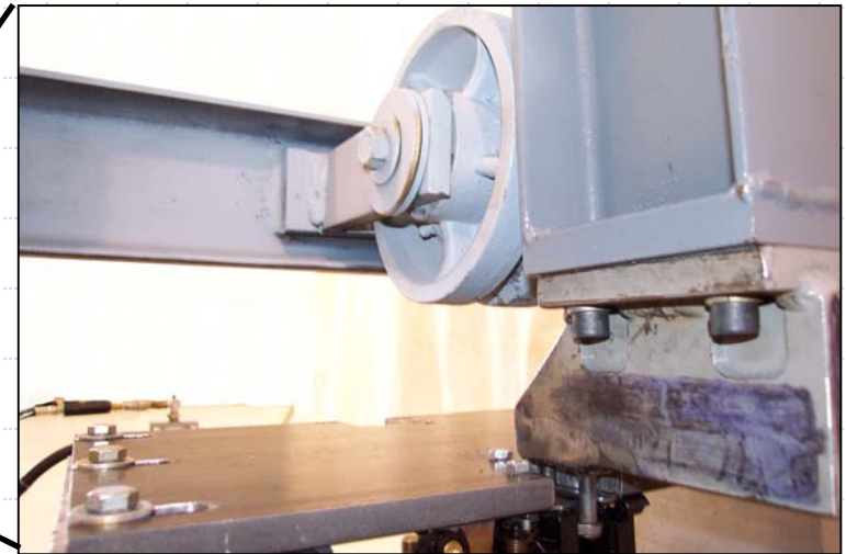
Striker attachment to loading device
