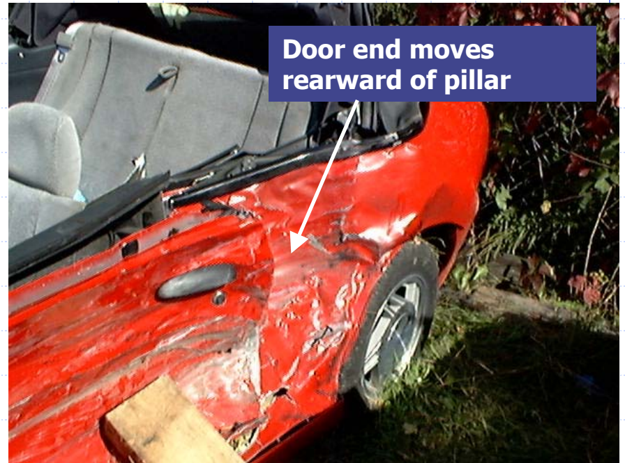
Evidence of rearward displacement of the door
