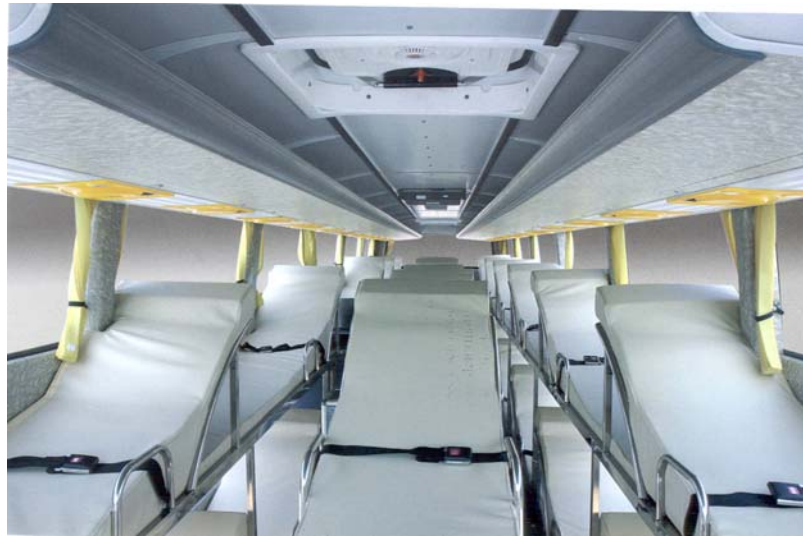
Fig.6. Two levels bed arrangement with two gangways
