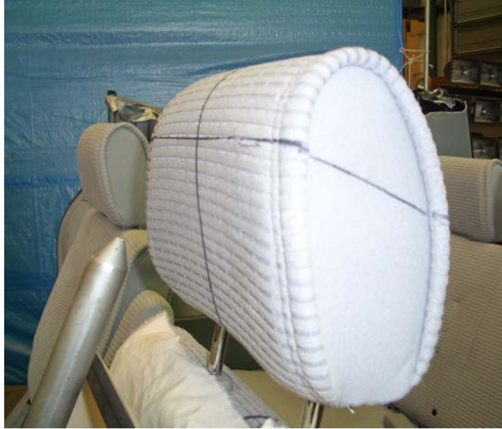
Figure 7 - Line indicating the plane 65 mm below the top of an adjustable head restraint
