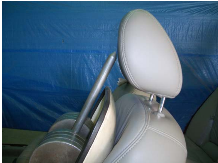
Figure 3 - Interference of head restraint with head room probe
