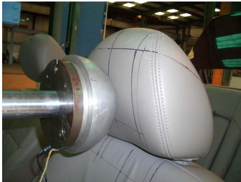
Figure 19 - Head form tangent to impact location (pre-test)
