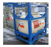
Reusable pressure tanks approved as tank containers or UN portable tanks with a filling capacity in the range of normally 500 to 5000 litres are increasingly being used in the industry, particularly for critical and high-value products. These containers may well be
