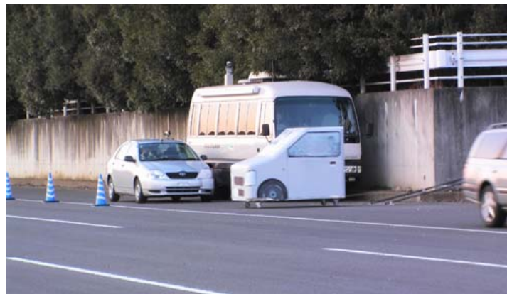
(a) Dummy automobile jumps out from the front left
