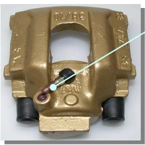
Thread of bleeder nozzle is greased with copper paste -> CU-lon-Reaction together with brake fluid. This can lead to accumulations in the brake system!
