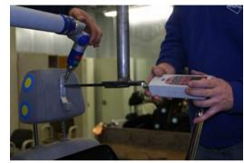
7. Repeat the above step (6) to determine the highest point that fulfils the requirement. Draw a horizontal line on the head restraint which goes through this point and crosses the vertical borders.
