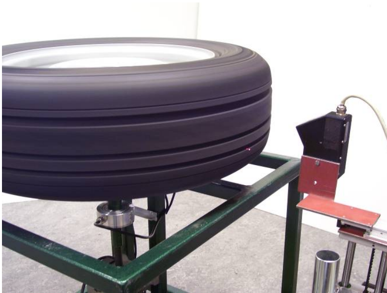
Shown profile scanner for C1 tyres, also used scanner for C3 tyres
