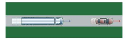
The advanced emergency braking system shall provide the driver with the warning specified in paragraph 2.2.3., when the test vehicle and the target vehicle are travelling in a straight line one behind the other with a vehicle centreline offset of not more than 0.5m under the following conditions;
