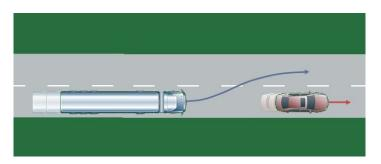
The advanced emergency braking system shall not react in any way when the test vehicle is approaching and passing the target vehicle at a closing speed of 10 km/h when both vehicles are travelling initially in the same lane. Each lane to be straight and 3.5m wide.
