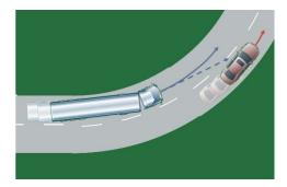
The advanced emergency braking system shall not react in any way when the test vehicle is approaching and passing the target vehicle at a closing speed of 10 km/h
