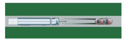
The advanced emergency braking system shall provide the driver with the warning specified in paragraph 2.2.3., and with the driver taking no action automatically apply the brakes<sup>2</sup> when a collision is inevitable.
