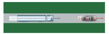
The advanced emergency braking system shall provide the driver with the warning specified in paragraph 2.2.3., when the test vehicle and the target vehicle are travelling in a straight line one behind the other with a vehicle centreline offset of not more than 0.5m under the following conditions:
