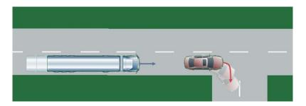
The advanced emergency braking system shall not react in any way when the test vehicle is approaching the target vehicle which is turning right in the case of a left hand drive test vehicle, or left in the case of a right hand drive test vehicle, from the direction of travel. The exit path travelled by the target vehicle shall follow a radius of curvature of between 10 and 20m.
