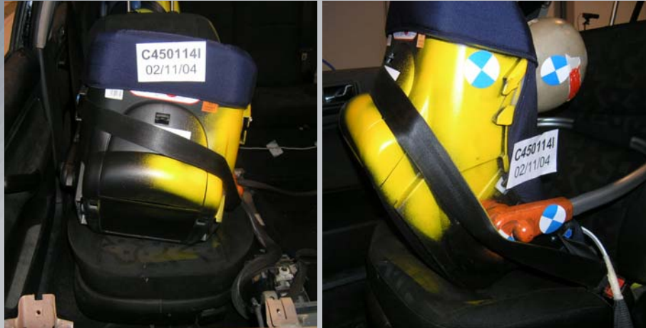
P3/4 on RF G0 seat (after test)
