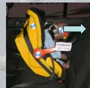
Neck tension in REAR impact
