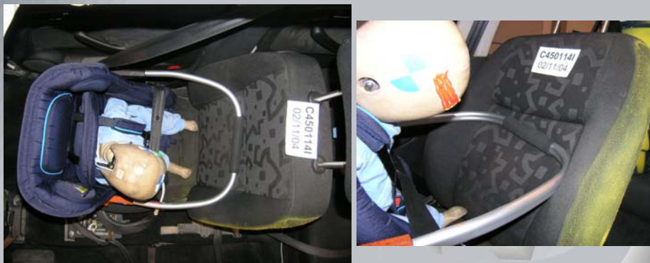
P3/4 on RF G0 seat (after test)
