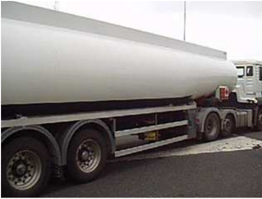
Three side direction indicators fitted to tanker note tanker rear lights obscured by semi-trailer.
