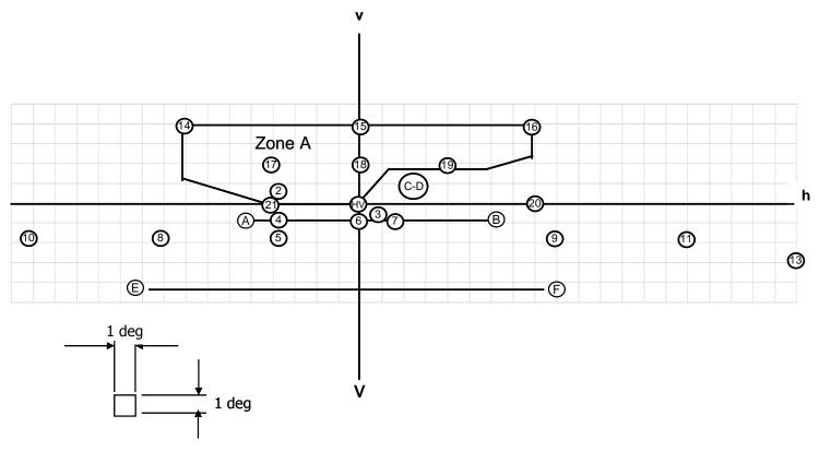
h-h : horizontal plane) passing through v-v : vertical plane) focus of headlamp
