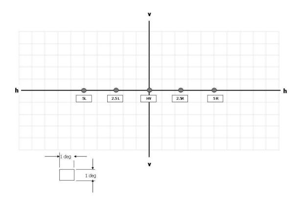
h-h: horizontal plane) passing through v-v: vertical plane) focus of headlamp
