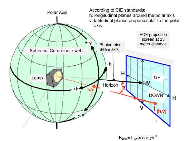
Figure B: Passing Beam for right-hand traffic
