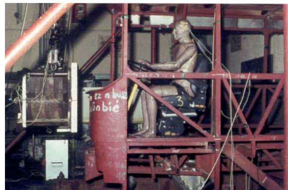
Fig.11. General arrangement of a pendulum impact test on a DC
