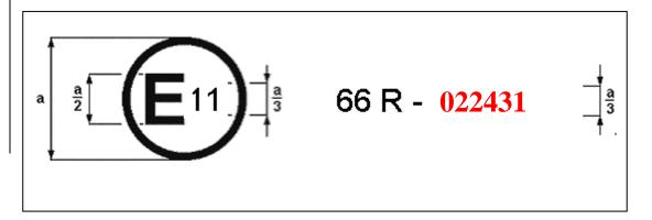
The above approval mark affixed to a vehicle shows that the vehicle type concerned has, with regard to the strength of the superstructure, been approved in the United Kingdom (E11) pursuant to Regulation No. 66 under approval number 012431022431. The first two digits of the approval number indicate that the approval was granted in accordance with the requirements of the 02 series of amendments to Regulation No. 66.
