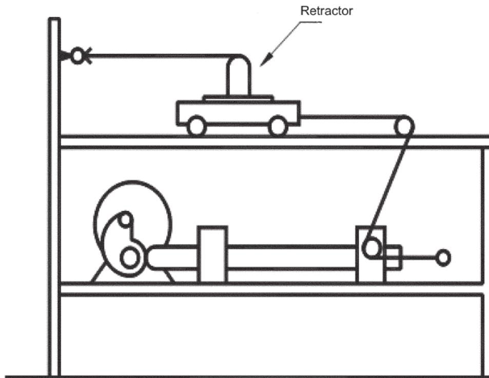
Set-up shows the configuration to test sensitivity on vehicle acceleration
