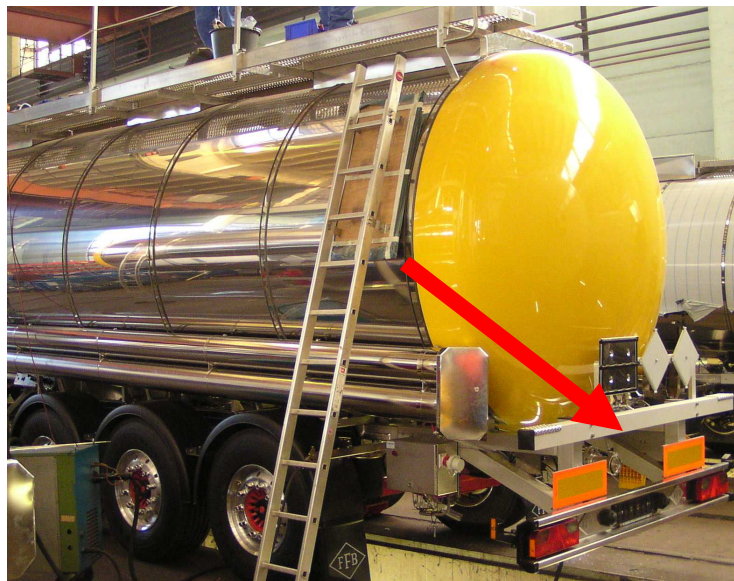
Fig.8: Rear protection in the form of a square tube
