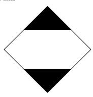
This marking shall be readily visible, legible and able to withstand open weather exposure without a substantial reduction in effectiveness. The top and bottom portions and the surrounding line shall be black. The centre area shall be white or a suitable contrasting background.
