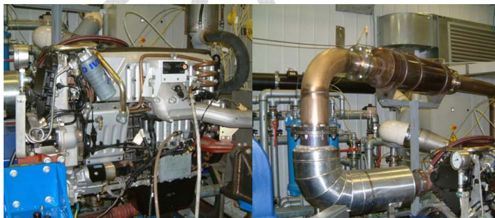
Figure 1: Typical Engine and Emissions Control System Installations
