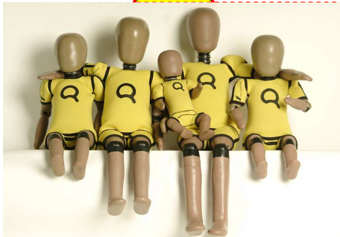
Q-dummy family from left to right: Q1.5, Q3, Q0, Q6 and Q1 [Q10 manikin being under development, not yet shown]
