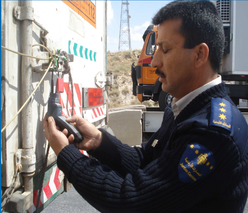
Attaching EDI Seal to a truck container at the Omari Border Crossing Point between Jordan and Saudi Arabia
