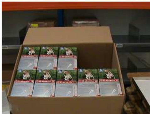
Picture 2: Filled with inner packages, which are wetted with a total amount 1.920 ml (after the last injection)
