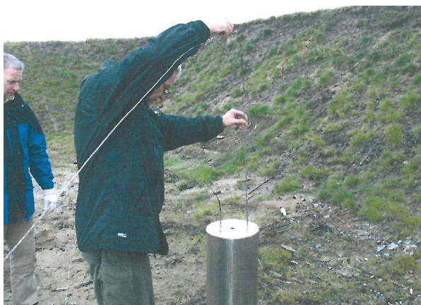
III. 3 Insertion of the thermo-elements to measure the temperature inside
