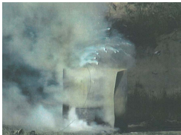
III. 8 Ejected melted substance, decomposing
