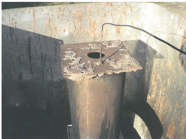
III. 13 Lid and wind guard with left-over substance at the bottom of the test set-up
