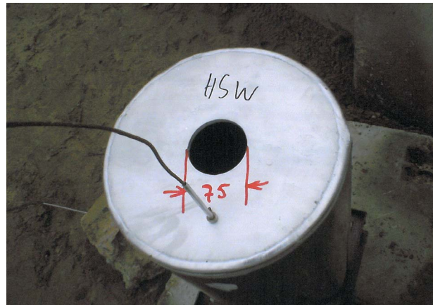
III. 5 Thermo-element for measuring the inside temperature
