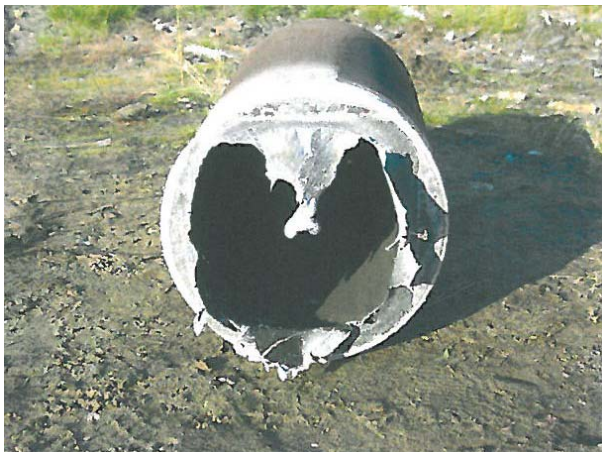
III. 15 Opened container bottom
