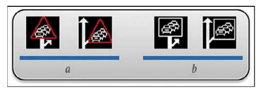
**Principle 18. Snow indication colours.** Four levels of driving/traffic are established associated with the condition of the road surface due to the presence of snow.
