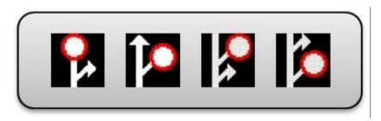
**Principle 17. Tailbacks.** Option «a» is established to indicate «tailbacks on the main road, alternative exit», or to indicate «tailbacks on exit, alternative main road». Option «b» develops the same concepts, but for the case in which the tailback is far from the VMP.
