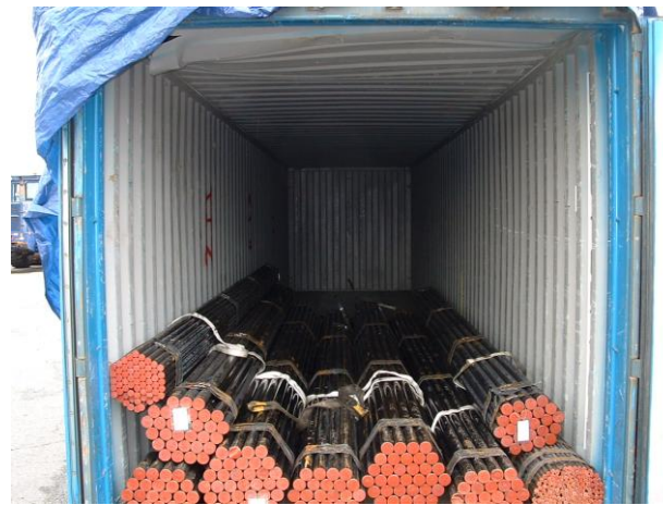
Figure 2.3. Unsecured steel pipe bundles
