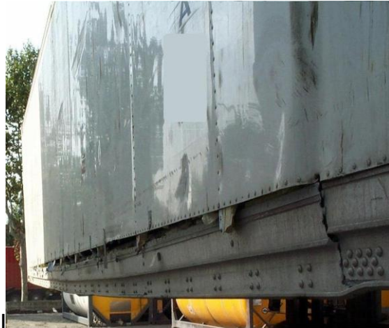
Figure 2.1. Detached bottom side rail
