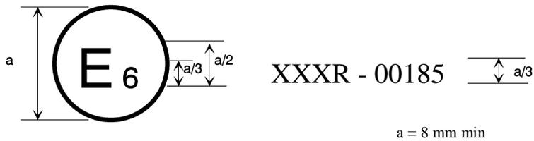
The above approval mark affixed to a vehicle shows that the vehicle type concerned has been approved in Belgium (E6) with regard to the AEBS-~~M~~ pursuant to Regulation No. AEBS-~~M~~. The first two digits of the approval number indicate that the approval was granted in accordance with the requirements of Regulation No. AEBS-~~M~~ in its original form.
