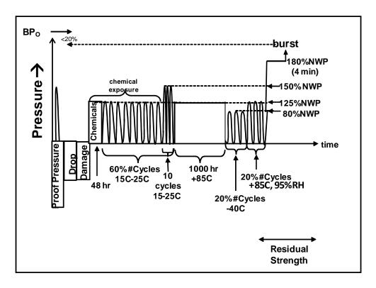
Figure B. 5.1.2 Verification Test for Performance Durability (hydraulic)
