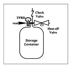
Figure A.3. Typical Compressed Hydrogen Storage System
