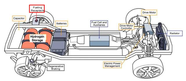
Figure A.2. Example of a Hydrogen Fuel Cell Vehicle
