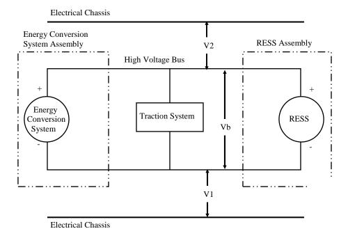
Figure 1: Measurement of Vb, V1, V2
