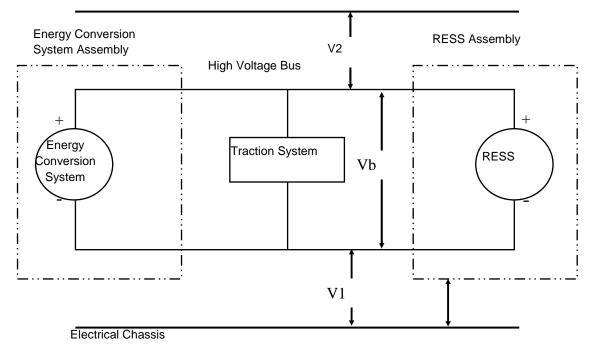
Figure 1 Measurement of Vb, V1, V2
