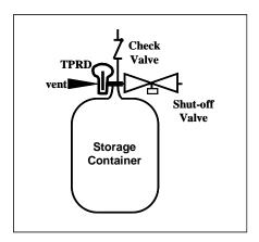
Figure B.5.1.1 Typical Compressed Hydrogen Storage System
