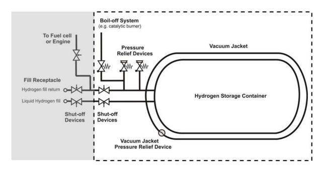
Figure A.4. Typical Liquefied Hydrogen Storage System
