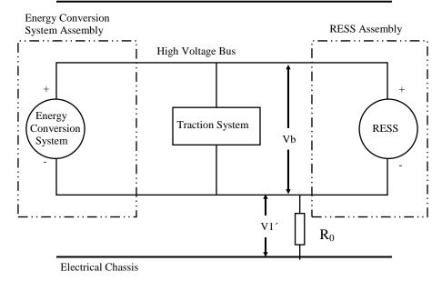
Figure 2: Measurement of V1'
