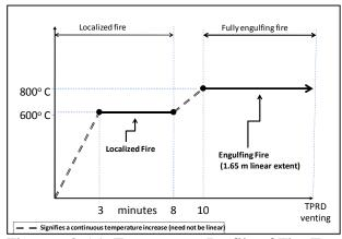
Figure 6.2.5.1 Temperature Profile of Fire Test
