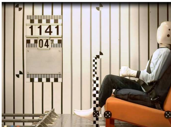
Figure 2a: Time 0 ms – Initial P10 dummy position
