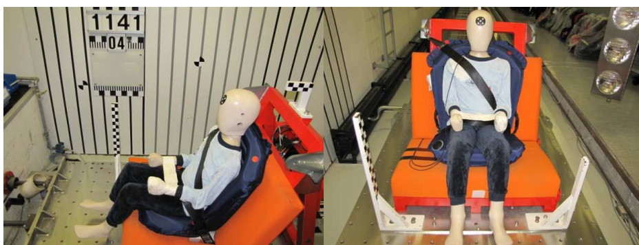
Figure 1: test set-up with the inflatable system
