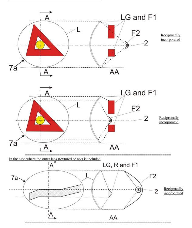
In the case where the non-textured outer lens is excluded, "7b" is the apparent surface according to paragraph 2.8 and F1 shall not be transparent to F2:
