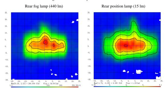
9. The simulation indicates that rear fog lamp has a maximum intensity of 266.8 cd and rear position lamp has a maximum intensity of 8.1 cd. According to the ratio of luminous flux of the two filaments, the maximum intensity of rear position lamp should be 9.1 cd, but it is simulated to be 8.1 cd. The reason is that the main filament is positioned and the second filament is not positioned in the focus of the reflector.
