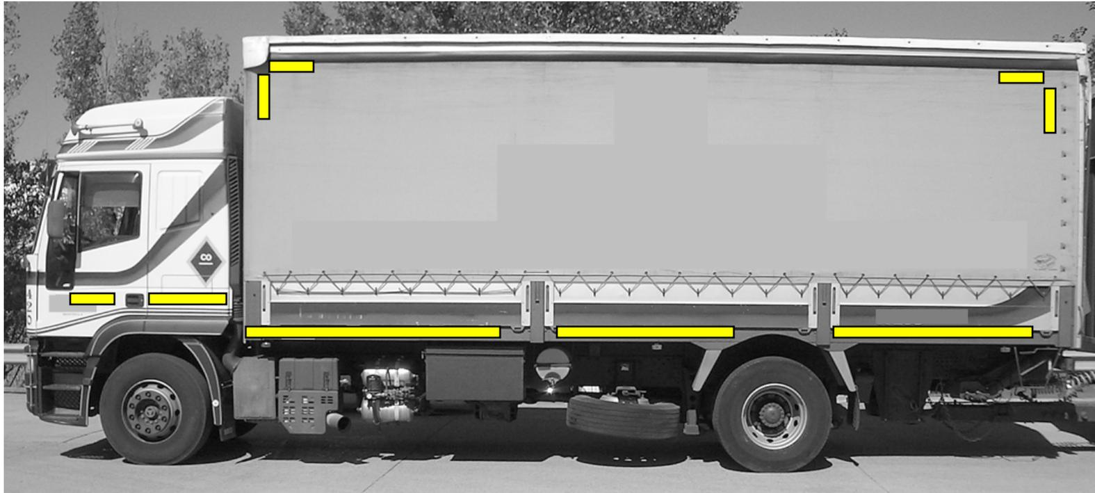
0.6 m    Cumulative horizontal length of marking: 80% of 7.2 m = **5.8 m**    0.6 m
