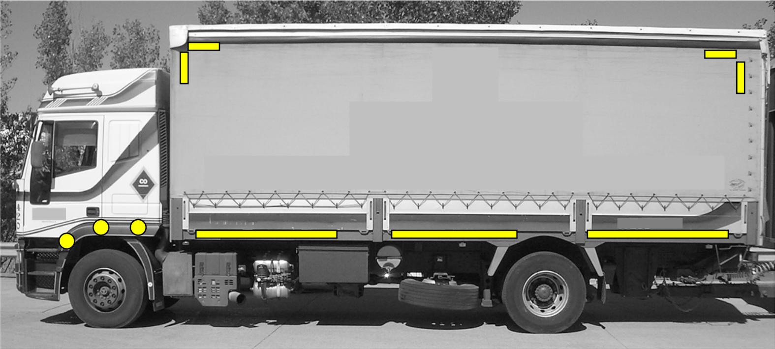
0.6 m      Marking = 80% of ,required length‘: 80% of 6.6 m = **5.3 m**      0.6 m
