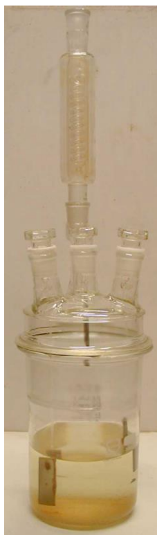
Figure 37.4.2: Exposure receptacle with reflux condenser
