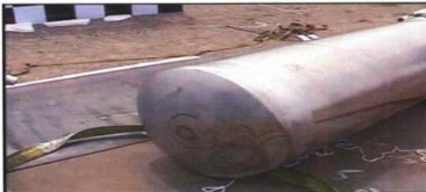
Figure 4: Tank Damage After 30 ft Drop Test
