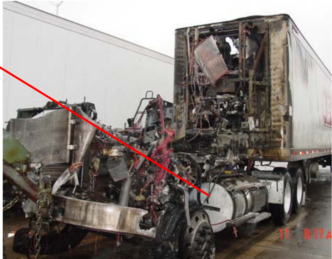
Figure 3: Complete melt down from other side. LNG tank
