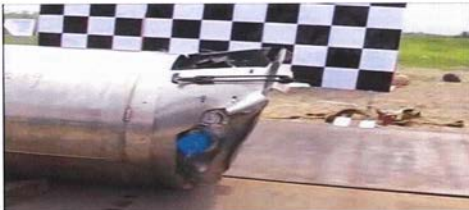
Figure 3: Tank Damage After 10 ft Drop Test
