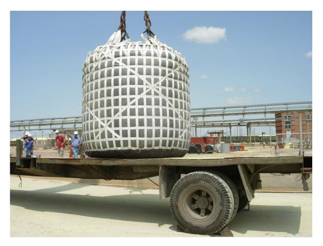
FBC was freely mounted on the truck platform. Tilting of platform with FBC and overturning prevention measures were carried out by 2 crane trucks of relevant capacity. The tilting angle was controlled by a digital inclinometer BOSH "DNM 60L". All testing procedure was shot by the photo/video camera CASIO Exilim "EX FH -100".
