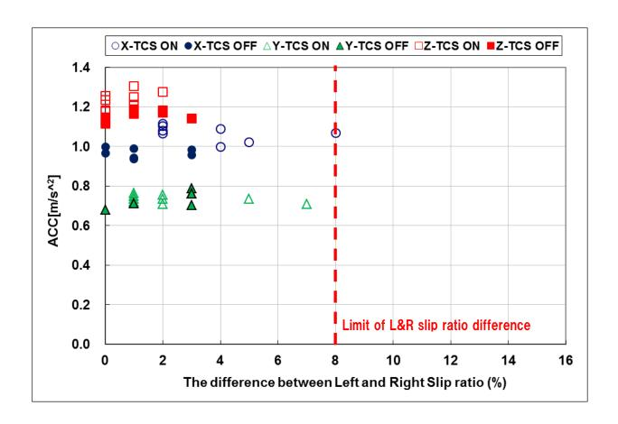
Using the Controlled Slip Procedure, it is possible to maintain the acceleration during the measurement without Traction Control System and Differential Lock.
