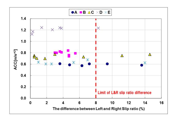
Acceleration during the measurement is stable even if the difference between left and right slip ratio is over than 8%.
